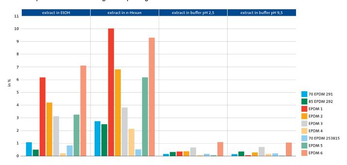
When the extraction values of black EPDM materials are compared, the two materials from Freudenberg as well as EPDM 4 are the clear winners in the benchmark comparison. Among the white materials, EPDM 253815 and EPDM 5 prevail. But the latter shows excessive extraction values in EtOH and n-hexane, and thus only EPDM 253815 is recommended overall. EPDM 4 also can not be recommended in general, as it shows a higher TOC value.
